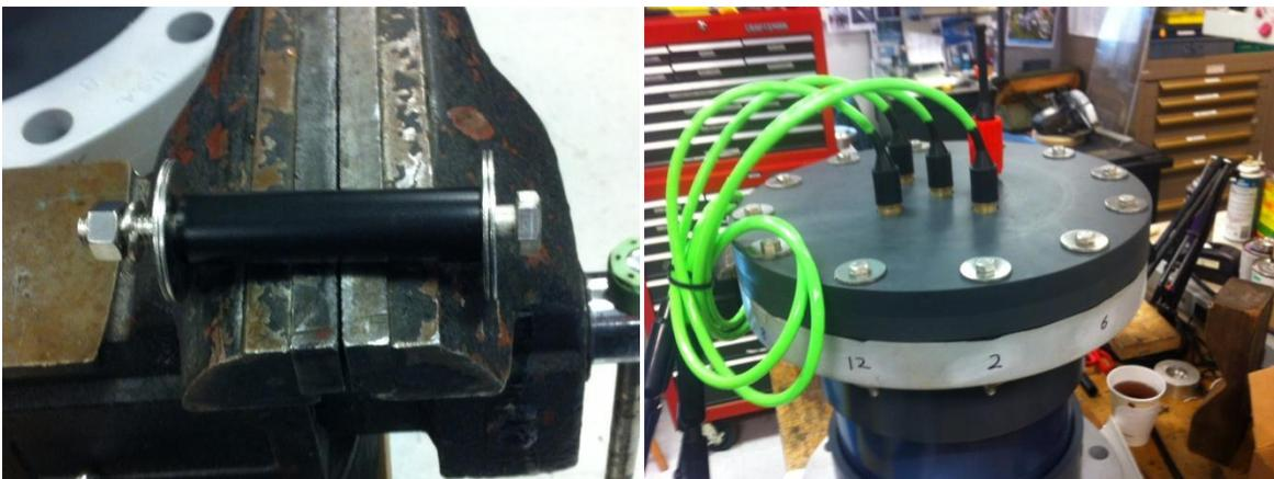
$\frac{3}{4}$ " spacers and Bolted ass'y with  $\frac{3}{8}$ " 316SS hardware, washers are doubled up for strength.
