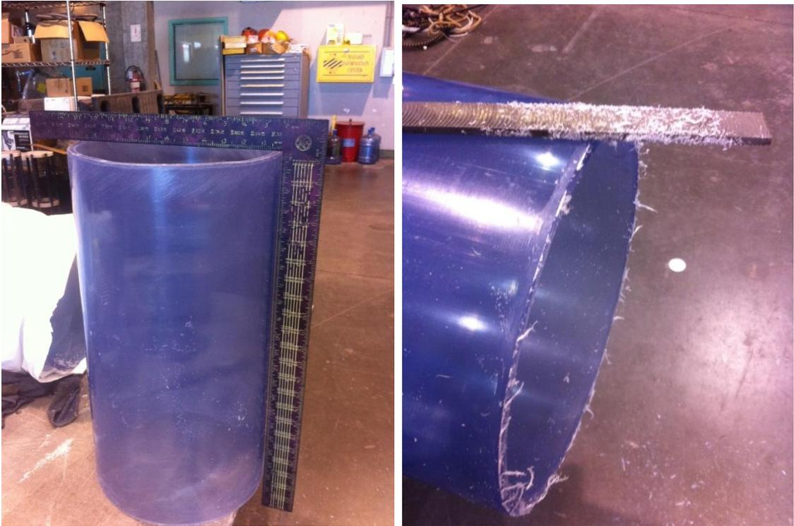
The Van Stone Flange inside bonding area has to be sanded and cleaned as well.
