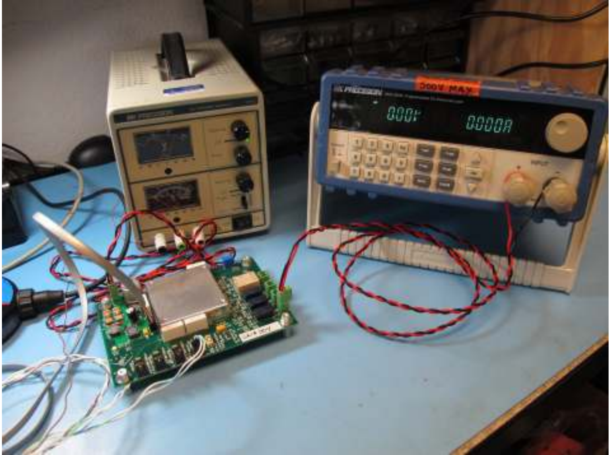
Figure 6: Load testing the SN board
