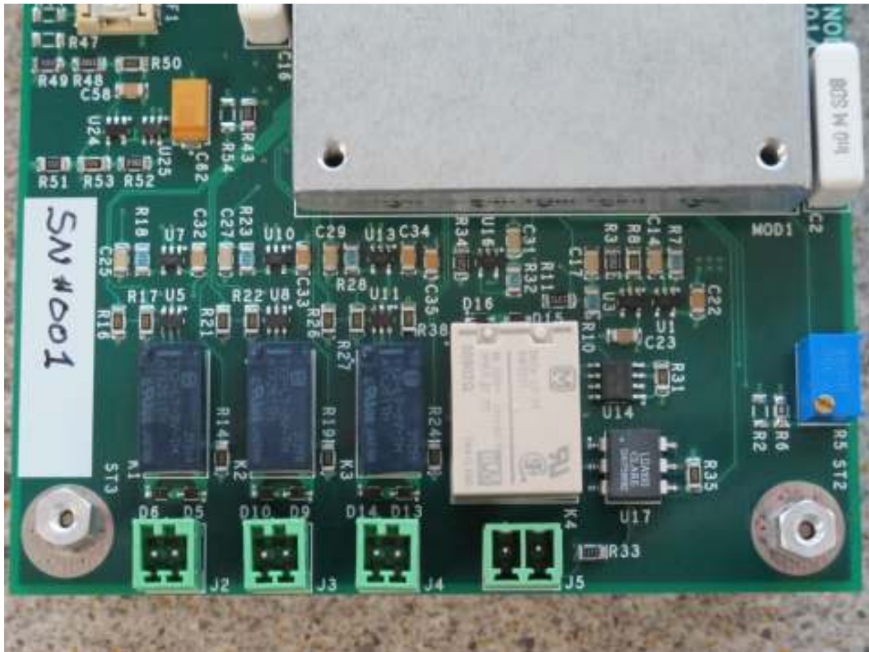
Figure 6: Output relays and connectors with trim circuit on far left (configured for trim up)
